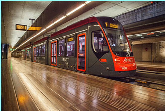
The Siemens Avenio Vehicle, shown in the Netherlands, the basis for the S70 now sold in the United States.
